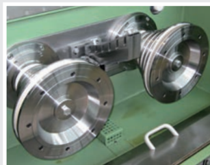
cone pair for thick wire Ø 3 mm
