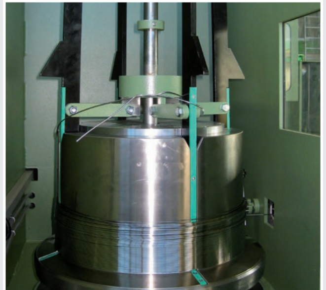
equipped with cone for coil manufacturing and stripper
