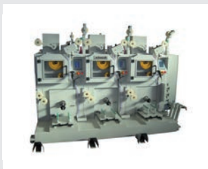
take up with calibration die and traversing spooler
