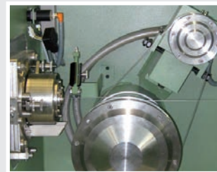
water cooled capstan and spreader dish, rotating final die holder
