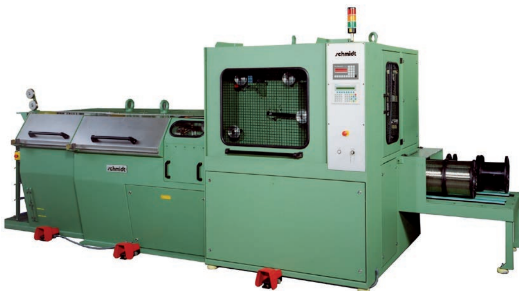
wet wire drawing machine type 150-40 with automatic spooler type A250-400
