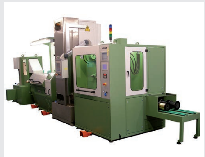
drawing machine with induction annealer and automatic spooler
