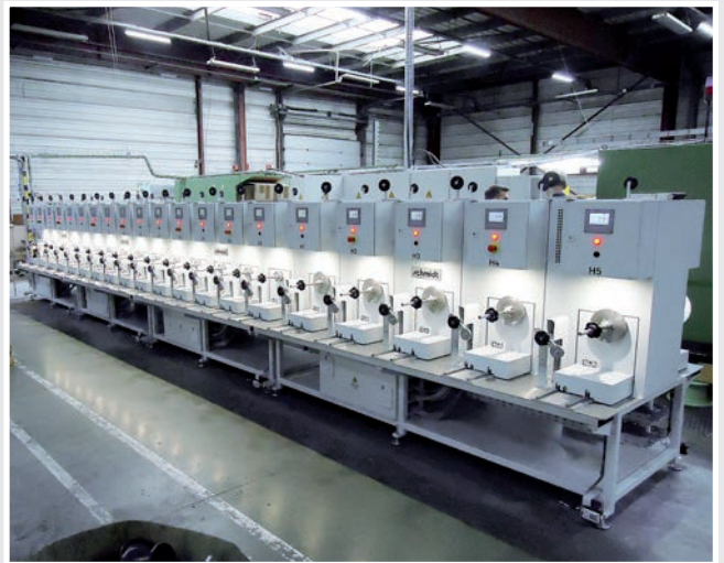
take up plant SD 20-30/40 for annealing process
