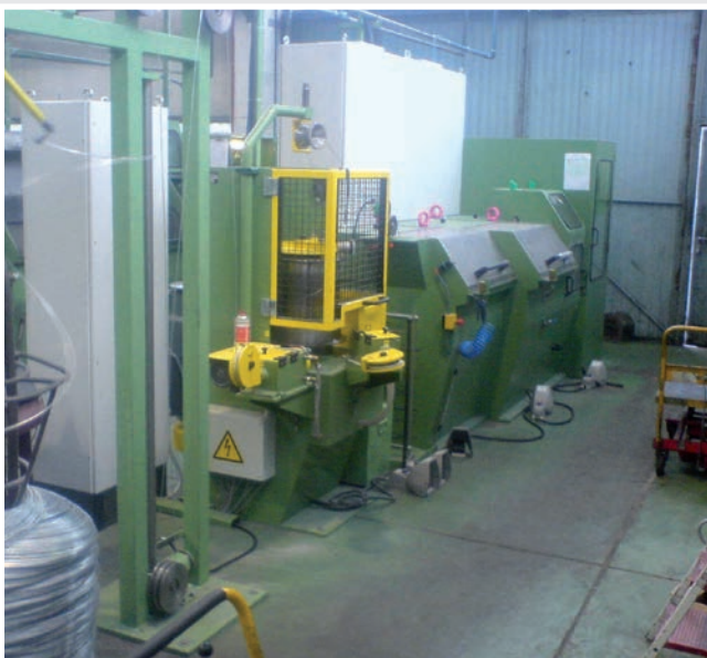
wet wire drawing machine type 150-40, inlet \varnothing 3,0 mm, with pre die and tail stock spooler
