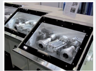
cone drawing machine with multiple drives for slipreduced operation
